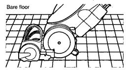
To prevent scratches or other damage to bare floors, Linoleum etc., press the agitator pedal to the "OFF" position.
